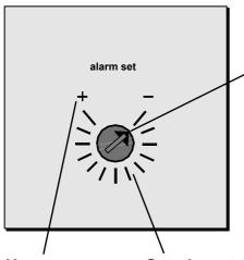
Upper temperature limit: Protection of unit and environment Set close to the switching point: Protection of the load
